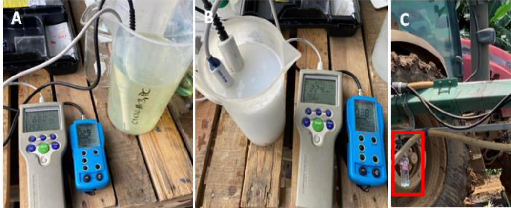
Figure.2A-C Measurement of the electrical conductivity of insecticide-nematicide solutions and nutritional cocktails. In both photos A and B, the device on the left is the conductivity meter and the one on the right is the peachimeter. C: the red rectangle shows the collection of the solution sample taken directly from the boom nozzle at the beginning and end of the application of each boom with a nutritional cocktail.
